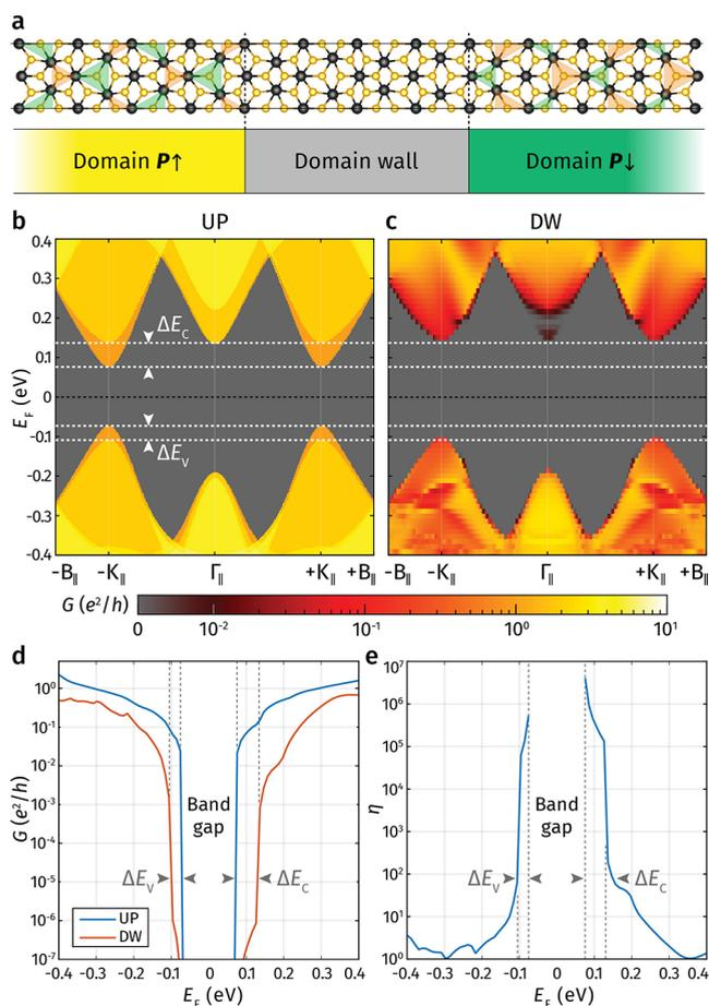
**Figure 4.** (a) *n*-VSV structure used for transmission calculations. (b, c) Conductance of the *n*-VSV in the UP state (b) and DW state (c) as functions of the Fermi energy  $E_F$  and electron momentum perpendicular to the transmission direction ( $k_{\parallel}$ ). Conductance is denoted by color, as shown in the color bar in the log scale. (d) Total conductance as a function of  $E_F$  for the UP and DW states. (e) ON/OFF ratio as a function of  $E_F$ .
